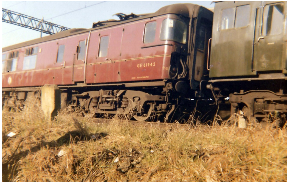
Car 61942 of two car Class 309 unit No. 309603 is seen in platform 5 at Colchester in February 1967: note the original maroon livery, the 'GE' prefix to the car number and the curved windscreens of the cab (David Reeve)
