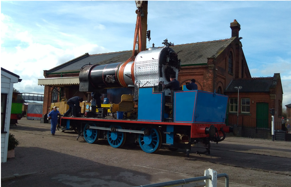
▼ Various Museum Members assist with the lifting of Number 54's boiler back on to the locomotive on 26th February 2017 - Peter Robinson
