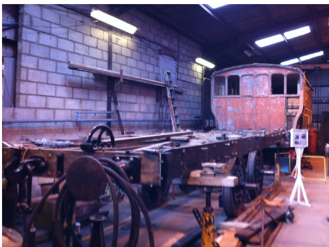
TB 308 - The chassis in the foreground and the body in the background, after many years of being used as a P-Way store on the bank next to Chappel North Signal Box
