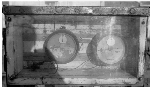
The repeater instruments for the signal arms, mandatory on distics and useful on others.
